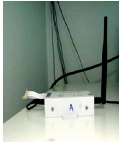
The edl-RF2 transmitter in position with its antenna.
