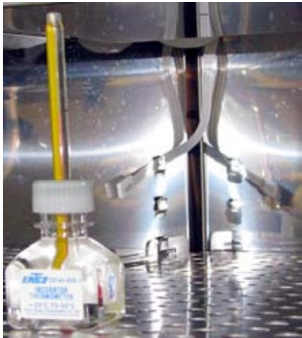
Position of the edl-RF2 probe and thermistor inside incubator.
