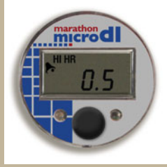
6. HI HR 0.5 shows alarm time hours over high threshold
