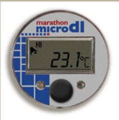
4. HI 23.1°C shows alarm has occurred and high temperature
