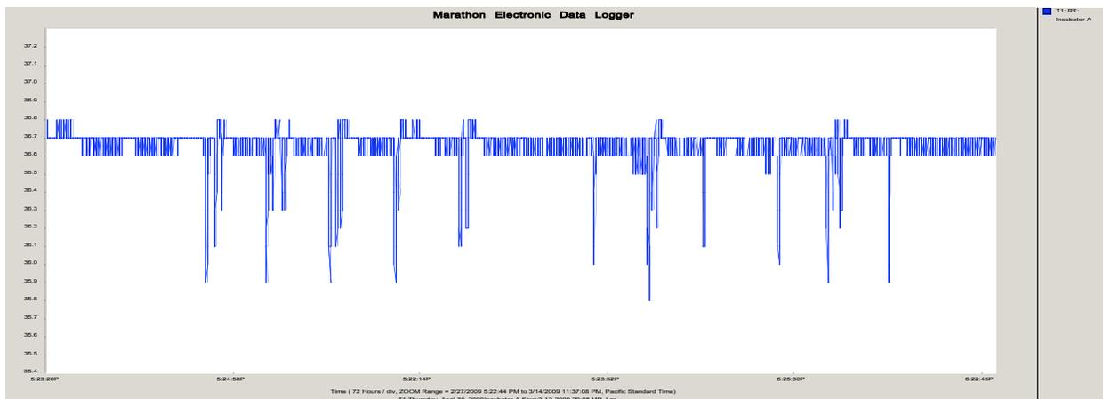
Incubator A showing temperature drops when the door was opened.
