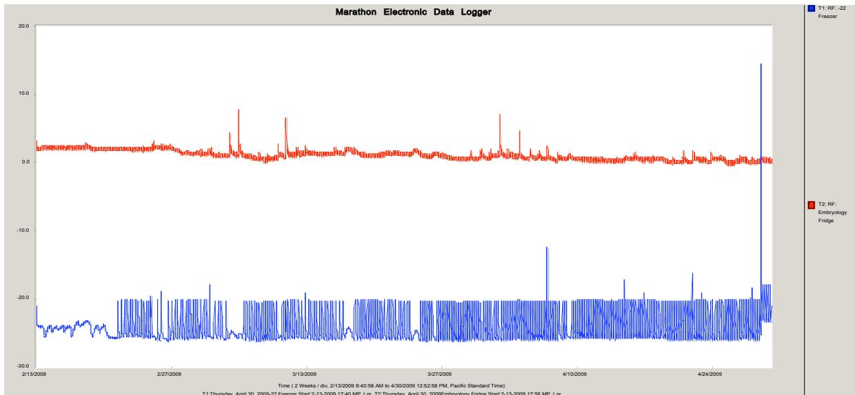
Internal temperatures of embryo refrigerator and freezer measured by edl-RF2
