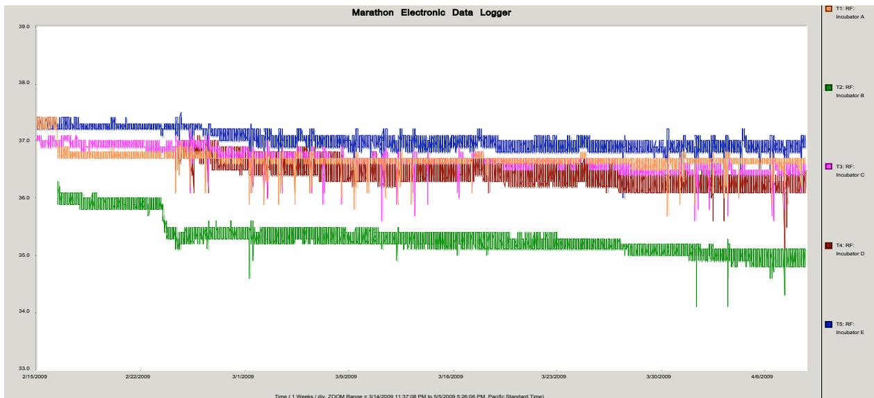
Internal temperatures of incubators measured every 4.25 minutes by edl-RF2.
