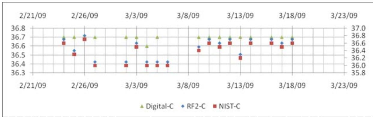
Comparison of the precision and accuracy of the edl-RF2 probes, NIST thermometers and digital display on the incubators.
